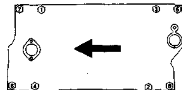
Fig. 36 Intake manifold tightening sequence—1997-98 engines
